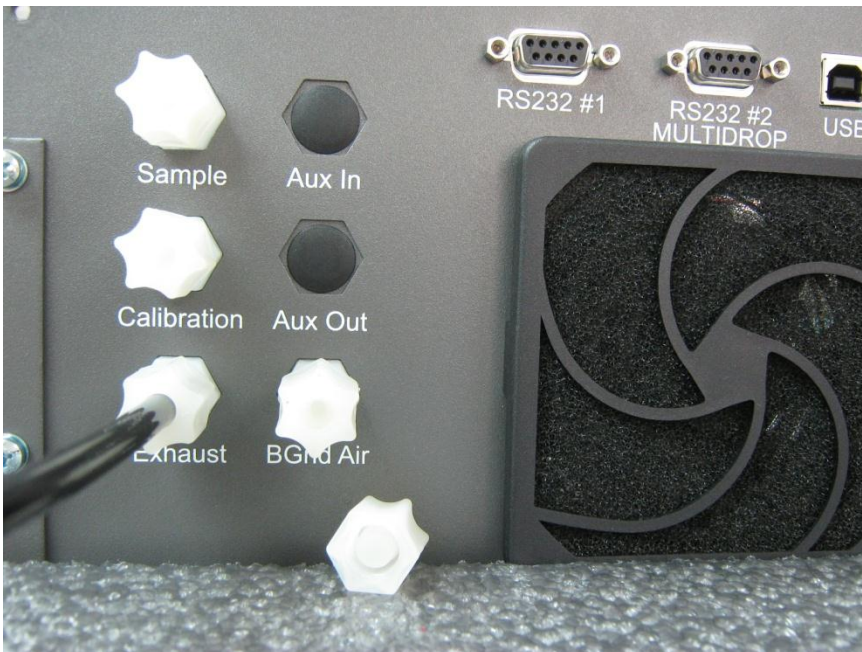
Figure 44 - Plugged sample, background, and calibration ports
