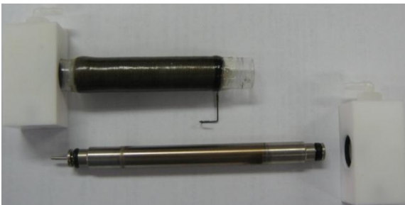
Figure 54 – Disassembled ozone generator cell assembly
