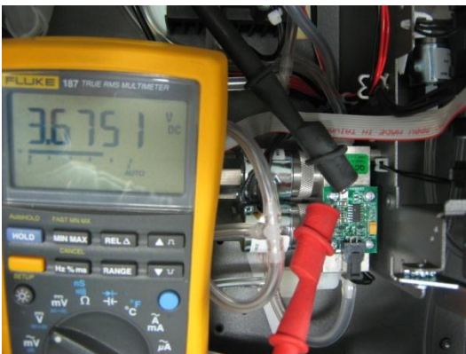
Figure 50 – Typical test point reading of manifold pressure sensor
