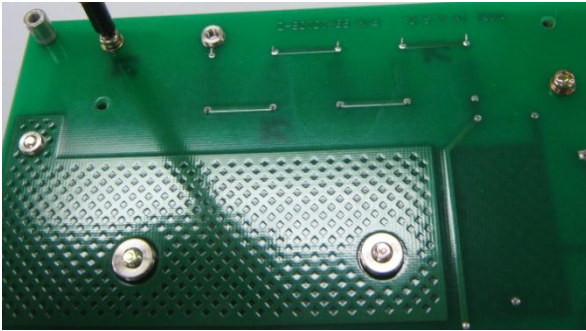
Figure 53 – Removing ozone generator cell assembly
