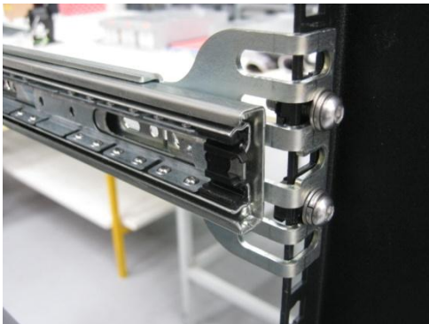
Figure 53 – Attach slides to front of rack
