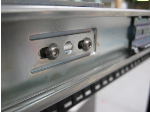
Figure 52 - Attach rack mount adaptors to outer slides
