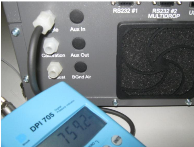
Figure 29 - Pressure calibration; external pressure meter
