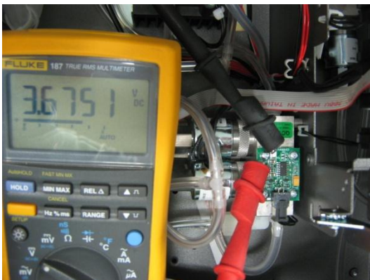
Figure 45 – Typical test point reading of cell pressure sensor.
