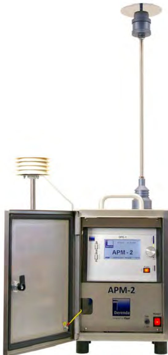
Figure 4: Overview of the overall APM-2 system
