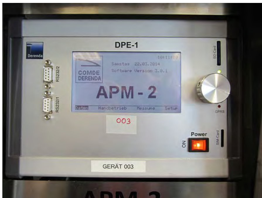
Figure 30: Front side of the APM-2 (top right side: SD-card slot, left side RS232)
