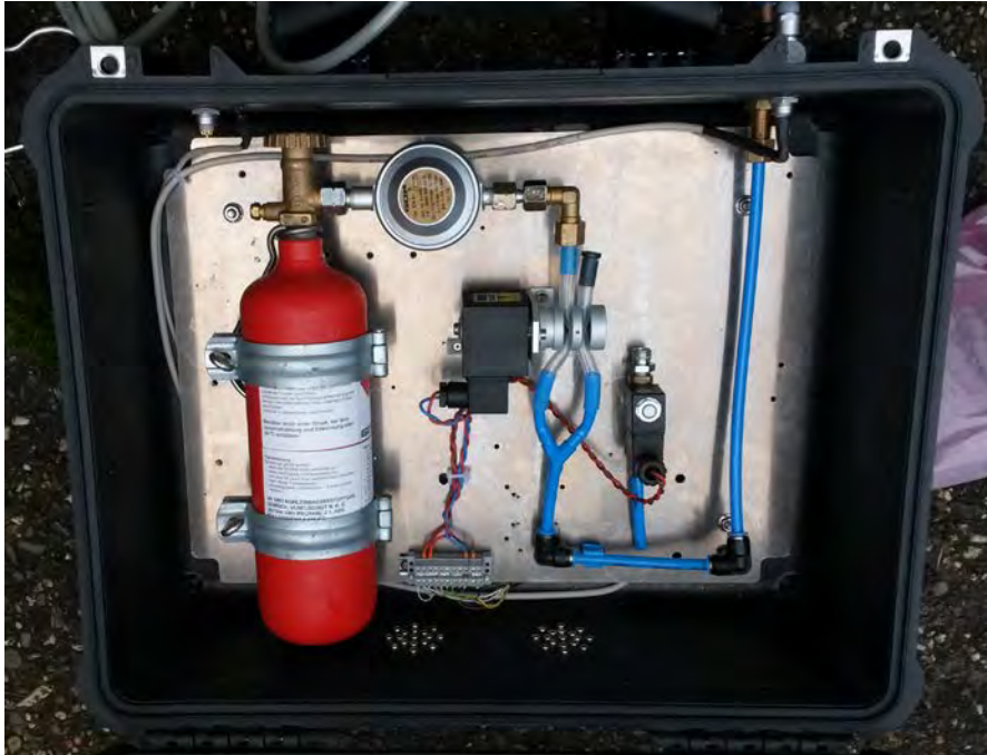
Figure 13: Test gas box for checking the sensitivity
