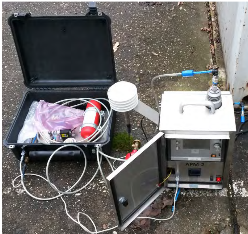
Figure 14: Test set-up APM-2 + test gas case
