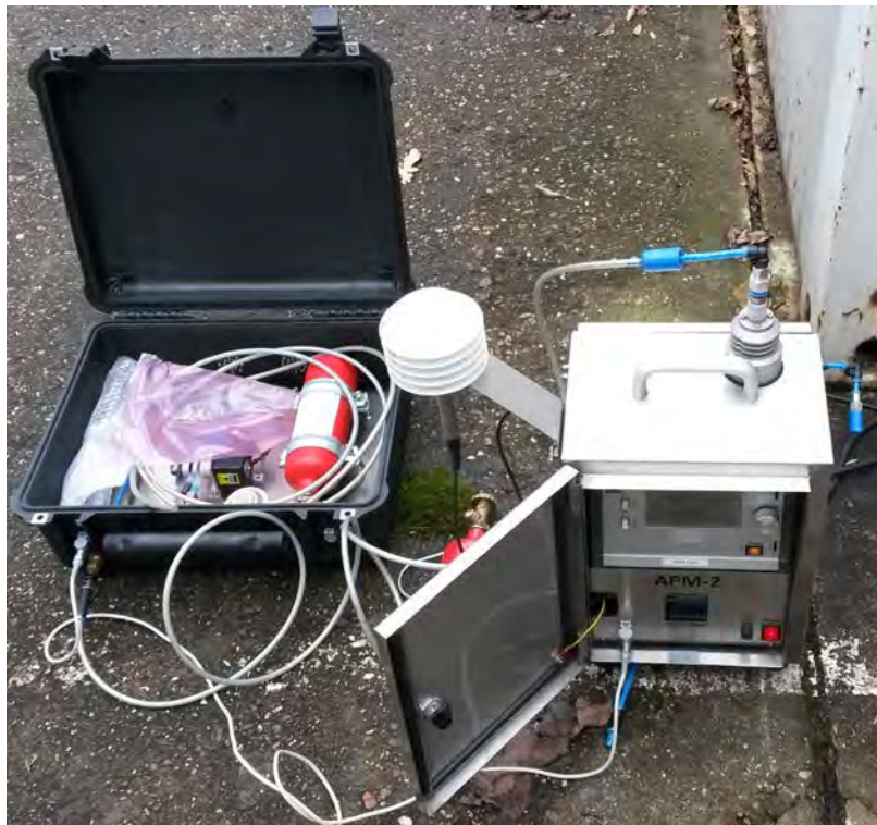
Figure 14: Test set-up APM-2 + test gas box
