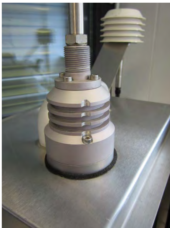
Figure 6: Virtual impactor for APM-2
