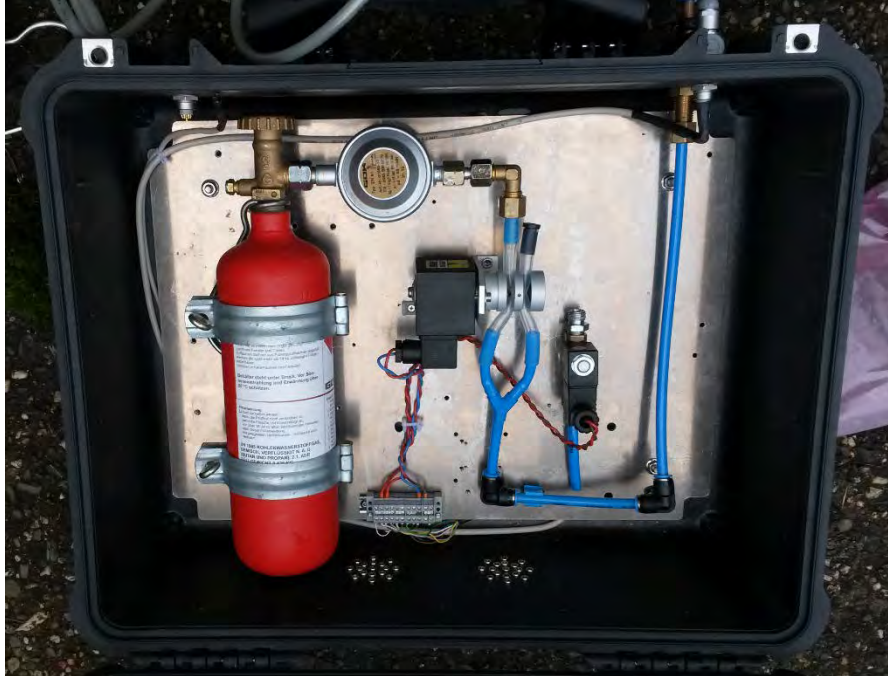
Figure 13: Test gas case for checking sensitivity
