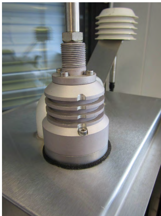
Figure 6: Virtual impactor for the APM-2
