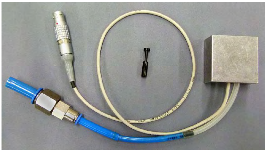
Figure 15: Test appliance for tightness check
