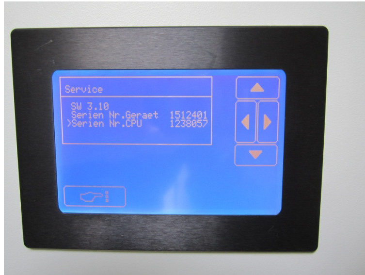
Figure 22: Display of software version – here 3.10 – in the menu “Parameter/Service/SW”
