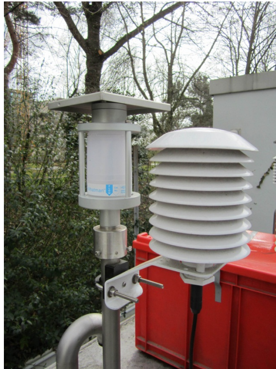
Figure 6: Zero filter for provision of particulate-free air, during field test
