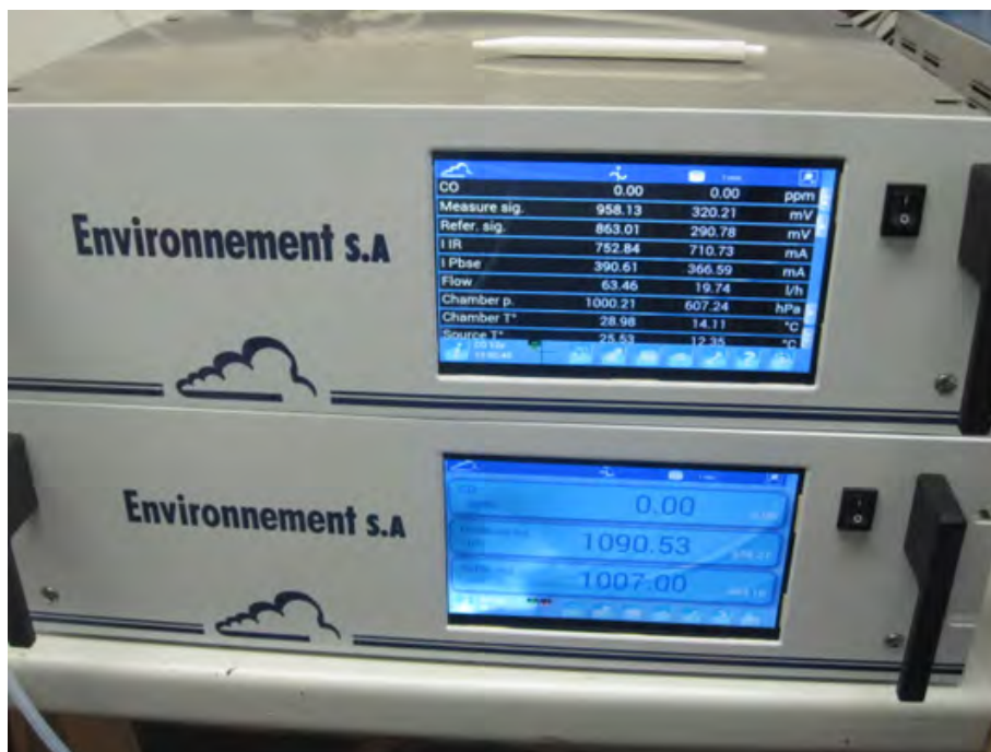
Figure 7: CO 12e test equipment
