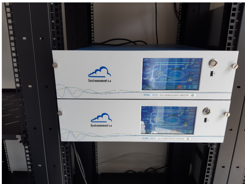
Figure 5: Tested VOC72e instrument with measured value display
