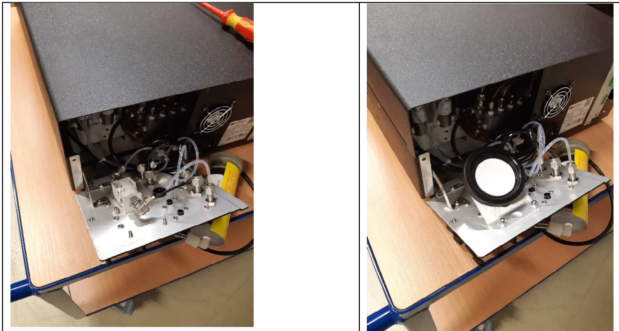
Figure 5: DFU filter (left) and 47 mm round filter (right)
